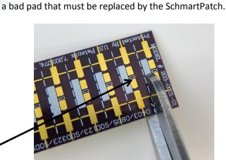
**Step 1** – Find the location on the PCB that you need to replace or add a component. The photo on the left shows
