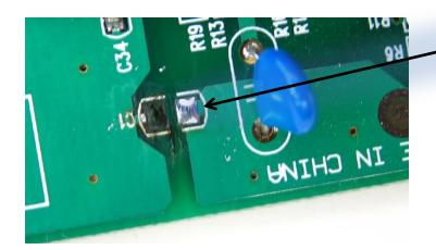
**Step 2** - With scissors or a blade, cut off one of the pads from the SchmartPatch. Cutting lines are silk screened on the Schmartpatch for your convenience.
