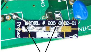
**Step 5** – Add jumper wires from the SchmartPatch to the correct points on your PCB.
