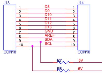
R5/R6/R7/R8: 0603 footprints for adding optional pullup resistors for I2C.
