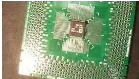
Hand Soldering a .5mm QFP Chip
