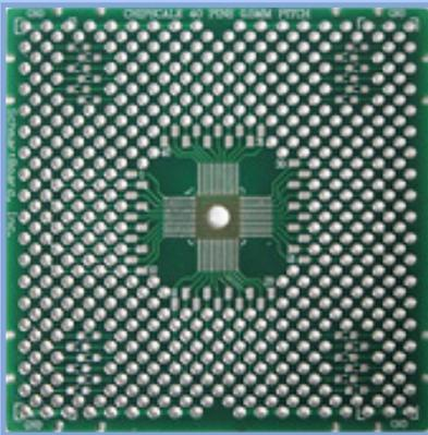
Schmartboard has released a new board for a popular component size, QFN 40, 5mm pitch. Some of the chips which use this board include: Linear Technology LTC3880, Renesas R2J20652ANP, Sensor Dynamics SM3255EN, ST Microelectronics STMPE16M31, STMPE24M31 & Texas Instruments: CC2531F128, CC2531F256, CC8520, CC8521, CC8530 & CC8531, TRF3761.
