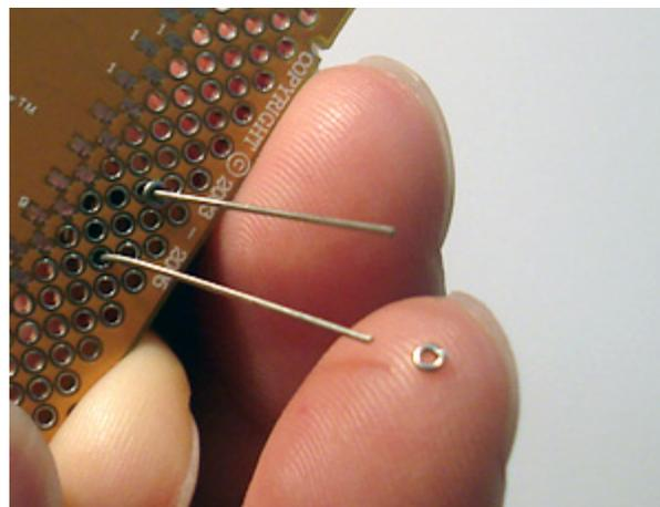
SchmartSolder are loops of solder produced in just the right diameter to fit over the component leads. One places the solder over the lead and flush to the circuit board and simply touches the soldering iron to the SchmartSolder. The SchmartSolder quickly melts and flows into the hole. The result is a perfect, neatly soldered component with no cold solder joints or other flaws.
