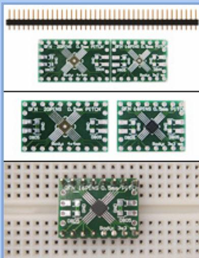
The first new board is a .5mm QFN/QFP to DIP Adapter. Included in the package are .5mm pitch adapter boards for 12 leads and 24 leads. The second new board is a .5mm QFN/QFP to DIP Adapter. Included in the package are .5mm pitch adapter boards for 16 leads and 20 leads. The third board supports both .5mm pitched 32-pin QFP and QFN devices.
