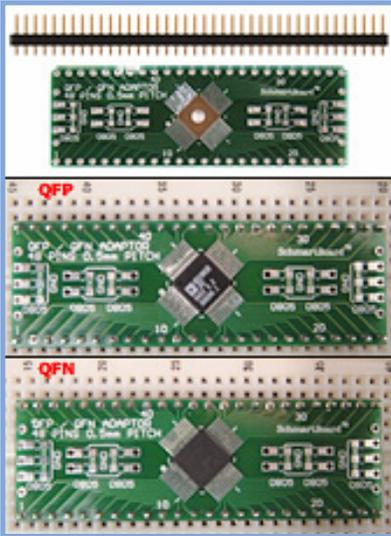
Breadboarders Arise! Today, your shackles are released as you no longer have to search for that elusive DIP version of components. Rise above your peers and use the IC of your choice. Create a breadboard circuit with an accelerometer in a QFN package, a microprocessor in a QFP package or a sensor with a .5mm pitch.
