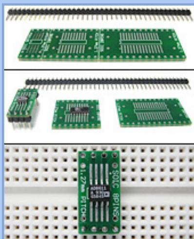
This product is an [SOIC to DIP adapter](#) with a twist. These have our patented "ez" technology which means that soldering the surface mount component is simple, and as with all of our "ez" boards, we are the only company with a patented solution for easily soldering surface mount parts.
