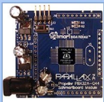
Our fully populated Parallax Propeller Development Board for only \$15.(Usually \$23) This board is populated with everything except memory and the optional Parallax Crystal. The Propeller chip makes it easy to rapidly develop embedded applications. Its eight processors (cogs) can operate simultaneously, either independently or cooperatively, sharing common resources through a central hub. The developer has full control over how and when each cog is employed; there is no compiler-driven or
