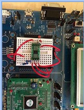
When using surface mount components on a breadboard, a SMT to DIP adapter is your best solution. For SMT to DIP adapters, only Schmartboard has "EZ" technology to make it fast, easy and flawless. Here is a perfect example of a project that might be more difficult without Schmartboard. The project is entitled "Real Time Clocks and Flash Memory".
