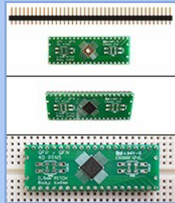
SchmartBoard|ez has released a new SMT to DIP adapter for 0.5mm Pitch 40 Pin QFP/QFN ICs.
