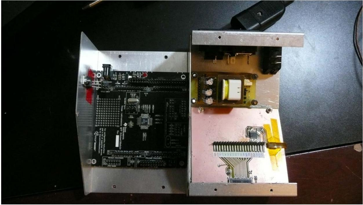
This is the inside of the controller. It contains a TRIAC with an insulated tab, allowing the use of the aluminum enclosure as a heat sink. On the right is the top half of the controller. It includes an LCD breakout board with a touch driver. The power supply is a simple mains transformer configuration. The board also contains the triac driver. For this application, I used a zero-cross detecting opto isolator to drive the main TRIAC.
