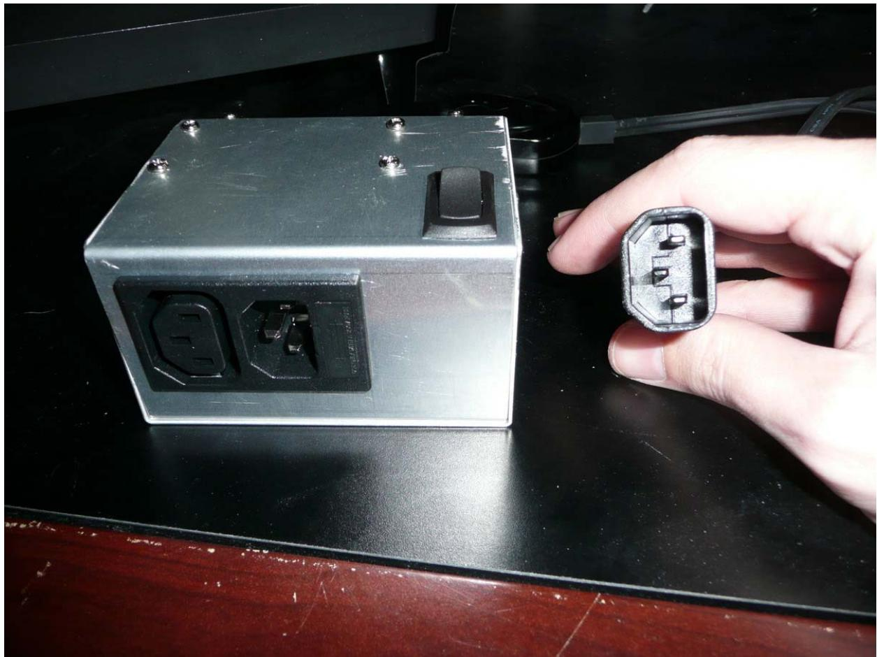
Here is the power outlet of the controller. Power travels in through the right plug and out through the left plug.
