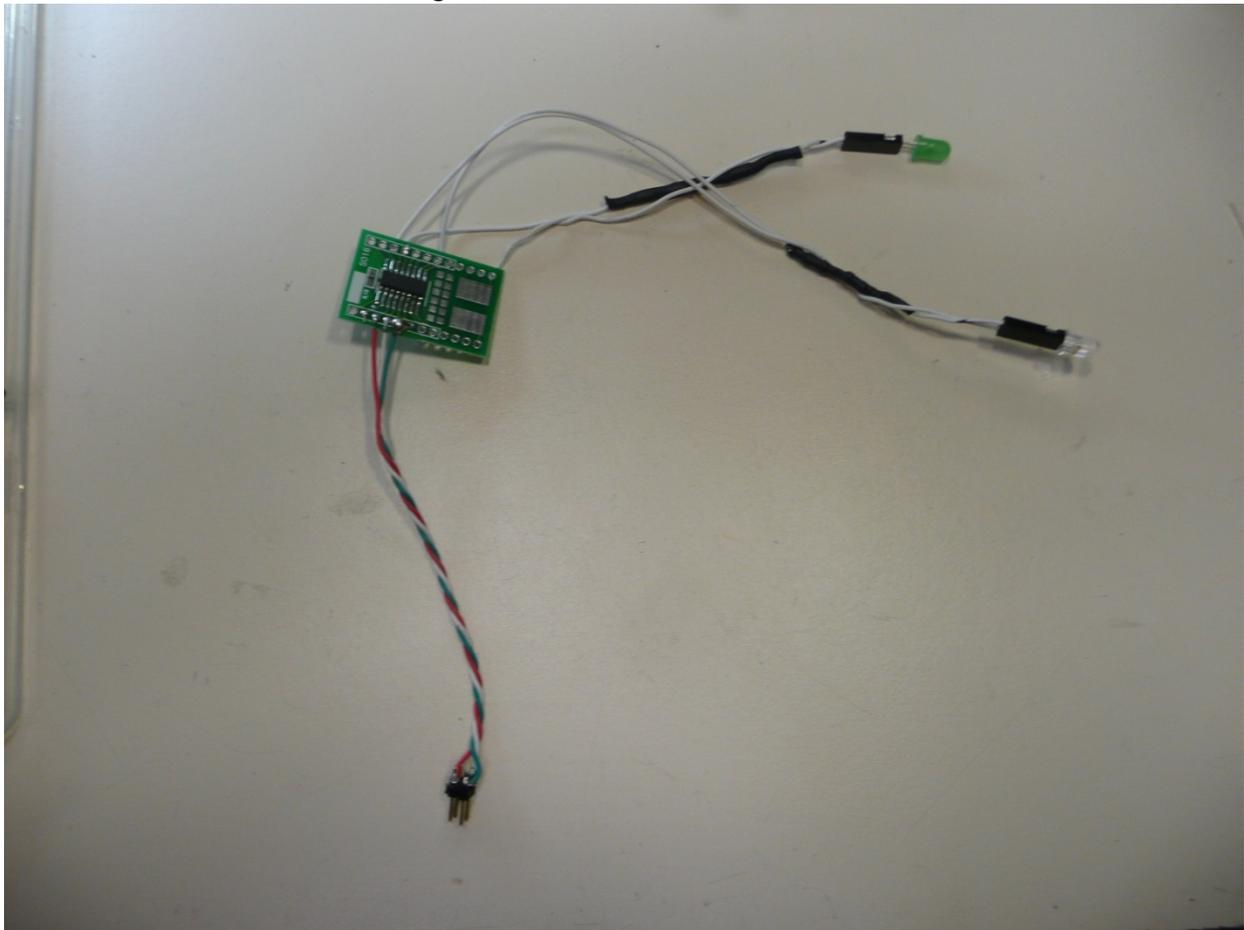
For Santa, a remote control pigtail (available from SparkFun) is controlled by the 1-wire device, as Santa requires full wall power to keep his reindeer moving.
