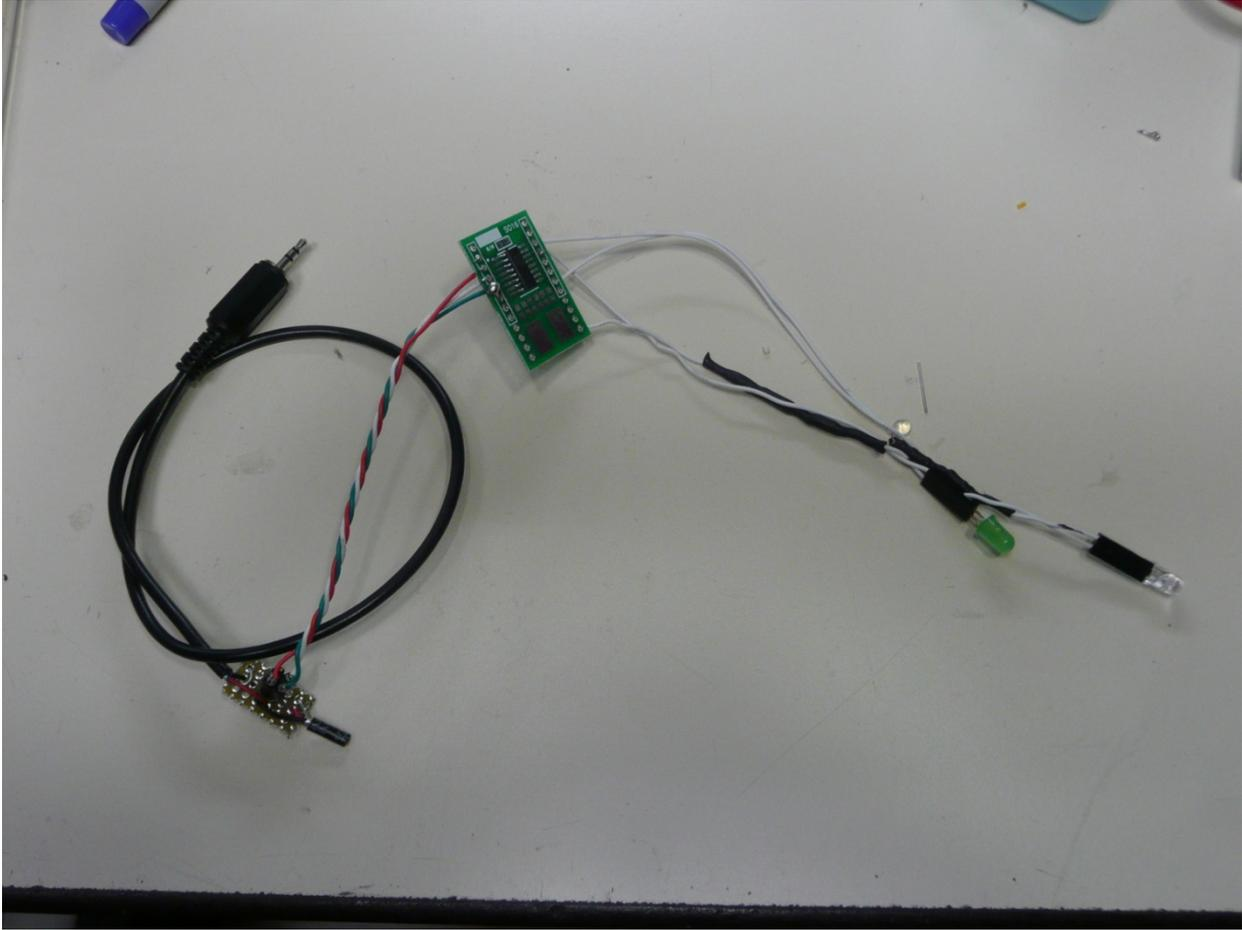
The main power and control board contains the voltage regulators, the main power control FET, the I2C – 1-wire bridge and mux chip, along with a header that connects to the MSP430 dev board. The power board contains two high power connectors that weren't required this year, and remain unstuffed. Likewise, the power control FET wasn't populated to make the debugging easier.
