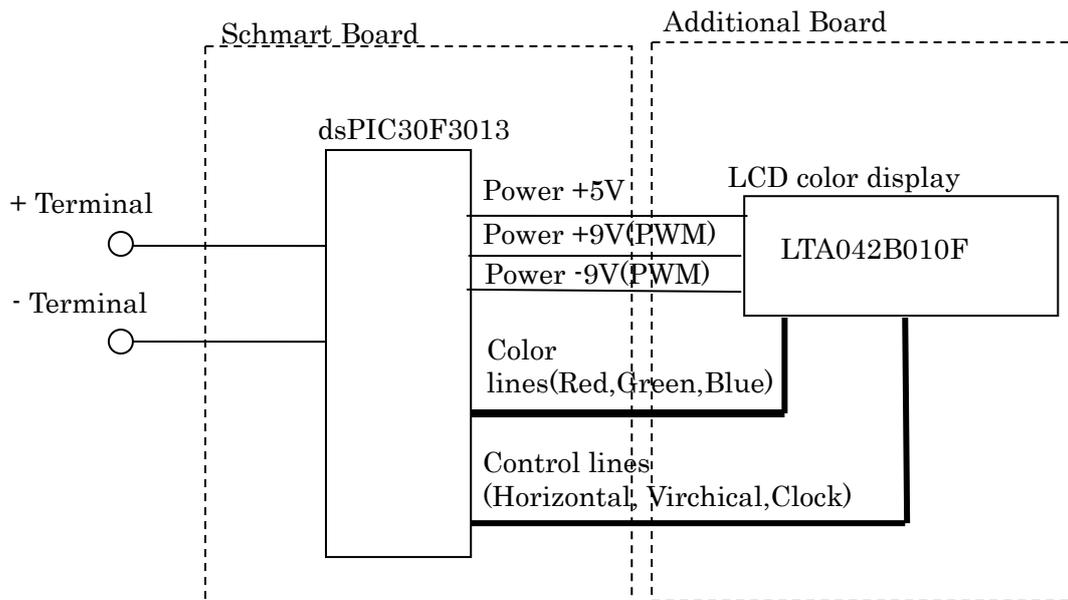
dsPIC30F3013 is mounted on SchmartBoard 8 Bit PIC Microcontroller Development SchmartModule board and connected additional board with 28 pin connector. LCD display is connected with 36 pin connector and flexible cable. So on additional board, 28 pin socket for SchmartBoard 8 Bit PIC Microcontroller Development SchmartModule connection and 36 pin connector for LCD display connection. Other parts such as input terminal or contrast voltage generator on additional board
