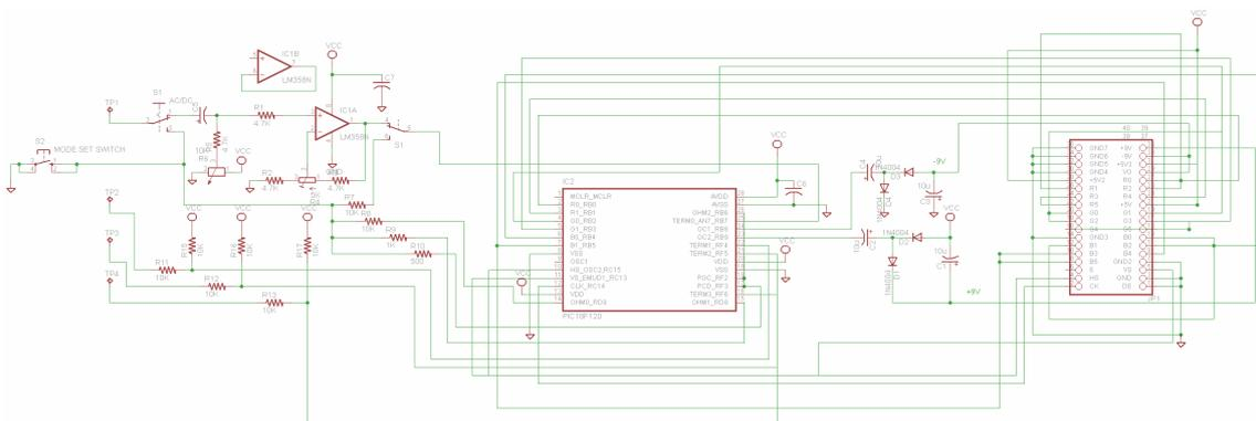
There are three parts. Input part, dsPIC30F3013 and LCD display LTA042B010F. dsPIC30F3013 is mounted on Schmart Board, input part and LCD display connector is mounted additional board.
