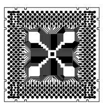
Support up to 100 pins QFP, TQFP, PQFP package IC with .5mm Pitch; 20 pcs. of 0603 package, and some thru hole passive components. 6 ground holes are connected a copper plane on the bottom side. A hole in the center gives access to a ground or thermal pad on IC.
