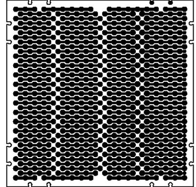
Through Hole 0.1" Spacing With Schmartboard's Signature 0.05" Offset Grid, 2" X 2"
