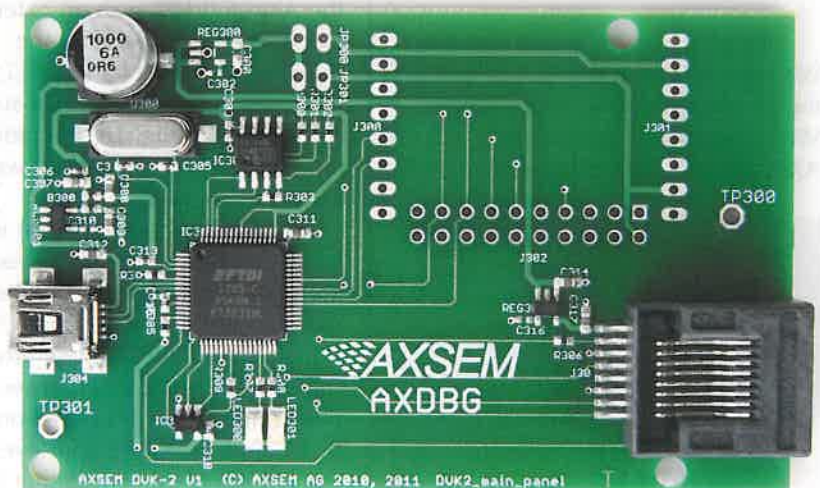
■ PHOTO 5. The AXSEM AXSDB debugger consists of an FTDI FT2232HL, a Microchip 93C46 EEPROM, a 12 MHz crystal, a couple of voltage regulators, and a single buffer IC.
