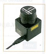
systems (AMHS). This scanner is an ideal solution to get a 2D or 3D (mounted to a servo or stepper) to map an environment. The unit essentially acts as the "eyes" for mobile robots for path planning and obstacle detection in unknown environments and needs only 100 ms to scan 240 degrees. The unit is lightweight, compact (50 x 50 x 70 mm), accurately measures distances between 60 mm to 4 m, and operates on 5 VDC via the USB port.
