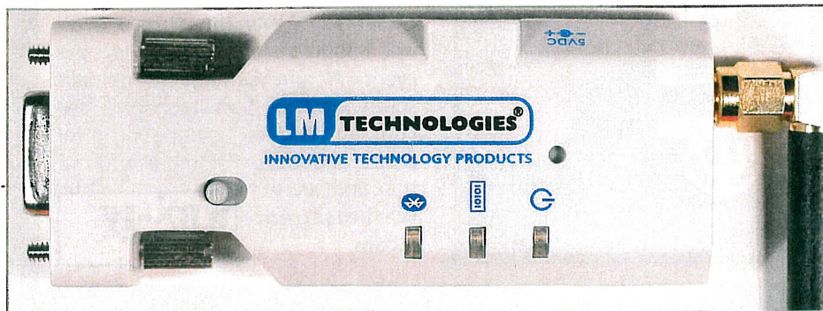
PHOTO 1. The nine-pin D-shell connector is intended to connect the Lemos Intl. Bluetooth radio module to the serial port of a personal computer. The external antenna implies that this unit is designed for long range communications. Note the +5 VDC USB power portal and the DTE/DCE switch in this shot.
