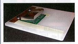
ntegrated Ideas & Technologies, Inc., has developed a prototype solder paste printing tool called the Desktop Companion II.
