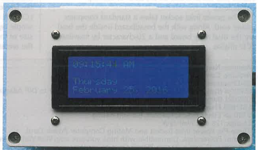
■ FIGURE 2. The LCD display mounted in the cover of the box.
