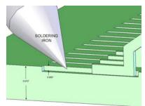
5) Remove the masking tape and repeat the steps 3 & 4 for other side(s) of the chip. Important Note: The tip of your soldering iron should be equal to smaller than the pitch of your chip. So a .65 mm pitch chip should be soldered with a tip equal to or smaller than .65mm. Failure to do this may potentially create shorts and damage the board.
