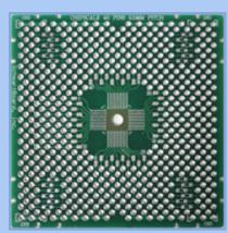
Schmartboard has released a new board for a popular component size, QFN 40, 5mm pitch. Some of the chips which use this board include: Linear Technology LTC3880, Renasas R2J20652ANP, Sensor Dynamics SM3255EN, ST Microelectronics STMPE16M31, STMPE24M31 & Texas Instruments: CC2531F128, CC2531F256, CC8520, CC8521, CC8530 & CC8531, TRF3761.
