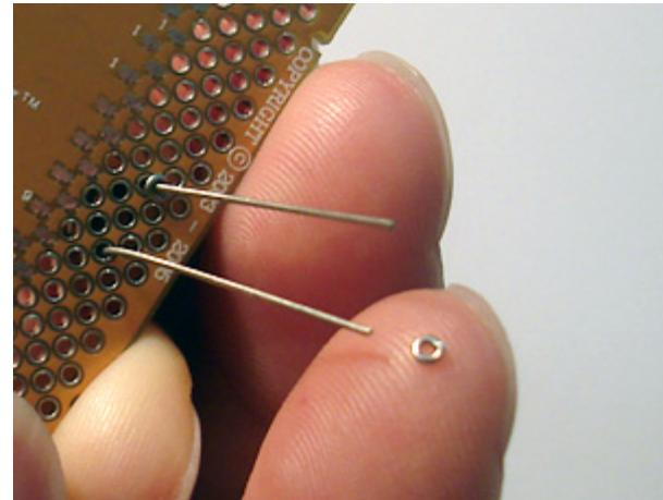
SchmartSolder are loops of solder produced in just the right diameter to fit over the component leads. One places the solder over the lead and flush to the circuit board and simply touches the soldering iron to the SchmartSolder. The SchmartSolder quickly melts and flows into the hole. The result is a perfect, neatly soldered component with no cold solder joints or other flaws.
