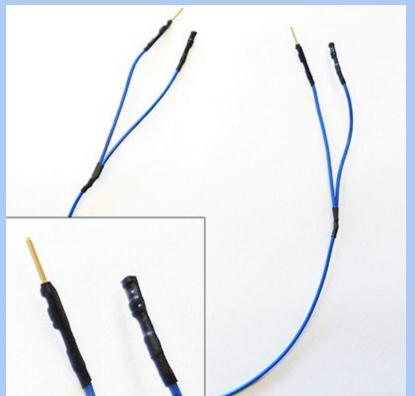
Based on input from users, we have invented a new type of jumper. It is a "4 Way Bus Jumper". The uses are many but in short it allows you to connect multiple points to a single common signal such as ground. It can also be used with electronic testing equipment such as logic analyzers as a signal interceptor to more easily access test points. These 11" jumpers will be available in 5 packs of Black, White, Red, Yellow and Blue sometime in August for \$9.00.
