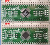
Breadboarders Arise! Today, your shackles are released as you no longer have to search for that elusive DIP version of components. Rise above your peers and use the IC of your choice. Create a breadboard circuit with an accelerometer in a QFN package, a microprocessor in a QFP package or a sensor with a .5mm pitch.
