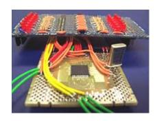
the "ez" technology. One of the sample circuits being displayed at the exhibit will be this Microchip based board that demonstrates multiple LED arrays. The board was designed and built by SchmartBoard user: Russell Pead of the Worcester Polytechnic Institute in Massachusetts. Our engineers were very impressed with the design.
