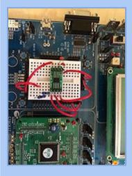
When using surface mount components on a breadboard, a SMT to DIP adapter is your best solution. For SMT to DIP adapters, only Schmartboard has "EZ" technology to make it fast, east and flawless. Here is a perfect example of a **project** that might be more difficult without Schmartboard. The project is entitled "Real Time Clocks and Flash Memory".
