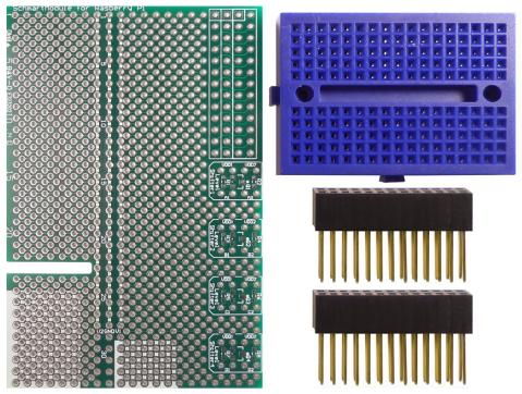
710-0010-27 SchmartBoard | ez .5mm Pitch, 16 Pin DFN Raspberry Pi Add-on Board Kit
