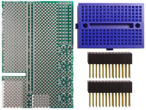
710-0010-27 SchmartBoard|ez .5mm Pitch, 12 Pin DFN Raspberry Pi Add-on Board Kit
