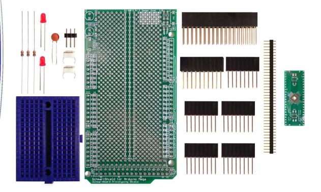
SchmartBoard | ez .5mm pitch 44 Pin QFP/QFN Arduino Mega Shield Kit
