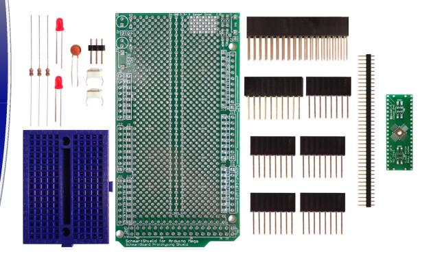
SchmartBoard | ez .5mm pitch 40 Pin QFP/QFN Arduino Mega Shield Kit
