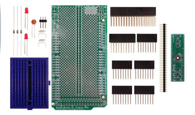
SchmartBoard | ez .5mm pitch 56 Pin QFP/QFN Arduino Mega Shield Kit
