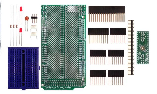
SchmartBoard | ez .5mm pitch 32 Pin QFP/QFN Arduino Mega Shield Kit
