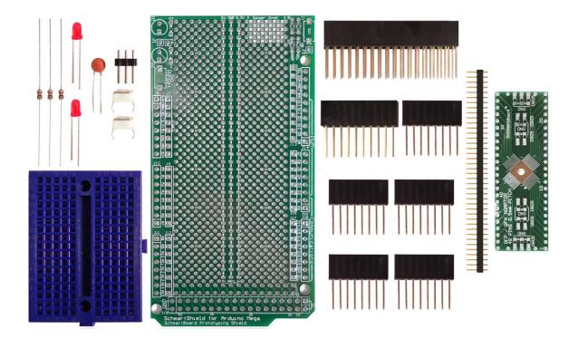
SchmartBoard | ez .5mm pitch 48 Pin QFP/QFN Arduino Mega Shield Kit
