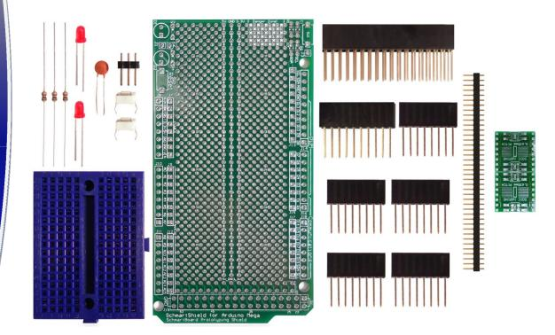
SchmartBoard | ez .635mm pitch SOIC Arduino Mega Shield Kit
