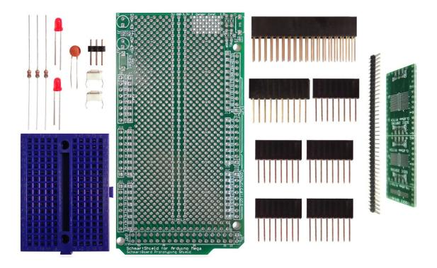
SchmartBoard | ez .65mm pitch SOIC Arduino Mega Shield Kit
